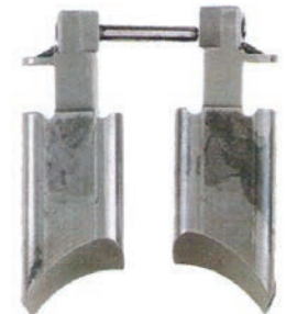
Power Valve Cleanliness Suzuki RM85 Motorcycle Field Test 40 Hours (1 Season Racing Circuit)
